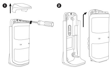
Remove the top cap and loosen screw (screw retained in wall plate).
